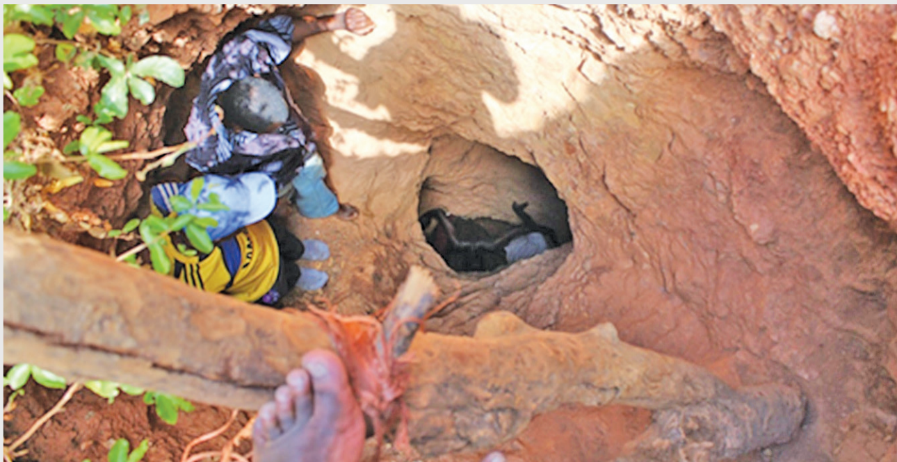
Chilubwa White Quartz Mine has 40 men working in an unventilated, unsupported tunnel that runs 10 meters deep (vertically) and 70 meters across the rock mass.
